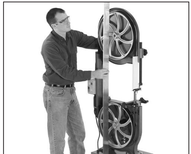
Figure 37. Checking wheel alignment with a straightedge.
